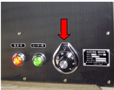
④ Sets a thermostat for 180°C
