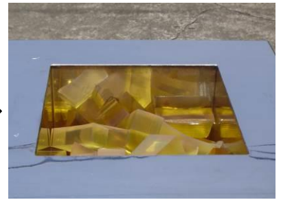
③ Put Seal Peel cut into pieces in a melting tank
