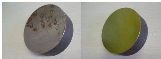
No coating → Rusting
