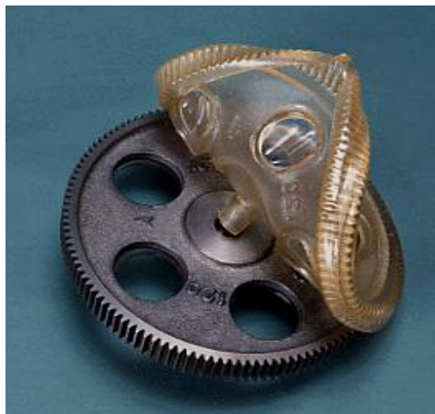
A gear can be easily peeled after keeping for 10 years
