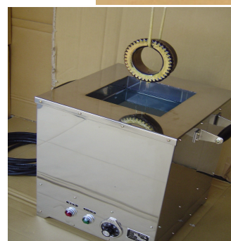
Sets a thermostat for 180°C It is possible to do preservation If drawing up slowly 60 seconds
